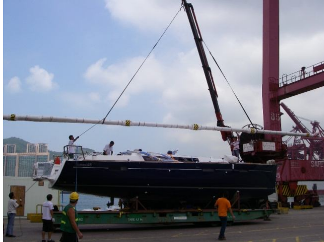
Unwrap, check, fit mast to roof
