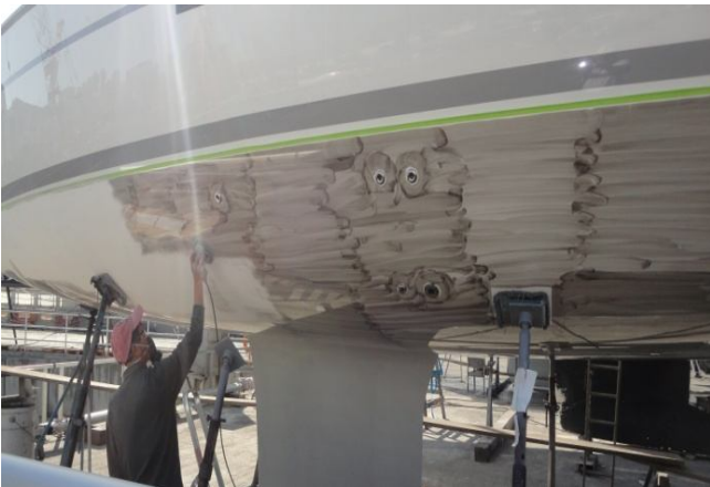
Marking then sanding of hull
