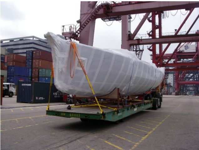
Boat arrives wrapped on RO RO Mafi trailer
