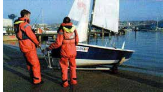
Hold the trolley by the handle and wheel the boat stern first into the water. 抓住船车把手，把船尾推入水中。
