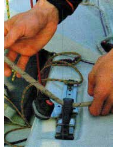
Step 2 Lead the jib sheets through their fairleads (guides for ropes). 第二步, 将前帆索穿过导缆孔(用于引导绳索)。
