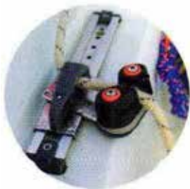
Jib sheet (rope) is led through a fairlead and held by a cam cleat. 前帆索（缆绳）穿过导缆孔，被（凸轮夹）夹绳器固定住。
