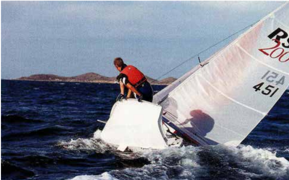
The point of no return for this dinghy crew. They are about to capsize during a gybe – probably because the centreboard is too far down, and they did not move their weight to the new windward side quickly enough as the boom swung across. 对这个小帆船船员来说已经没有回转的余地了。他们马上就要翻船了，这种情况发生在顺风转向的过程中，很有可能是因为稳向板放得过低了。并且在帆杆转动时，他们没有及时地转移到迎风侧。
