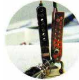
Shrouds hold the mast up and attach to the shroud plates. 侧支索保持桅杆竖直，下端连接在底座上。
