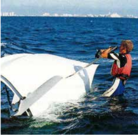
After inversion stand on the edge of the boat and lean back on the centreboard to bring the boat onto its side. 帆船倒置后，站到船边缘，抓住稳向板，身体后倾，使船回到一侧。
