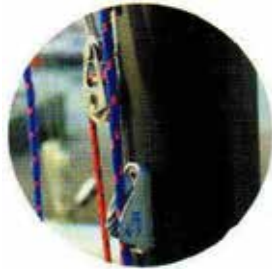
The halyard (rope) that hoists the sail is held by a clam cleat. 升降索（缆绳）用于升帆，被固定在夹绳器上。
