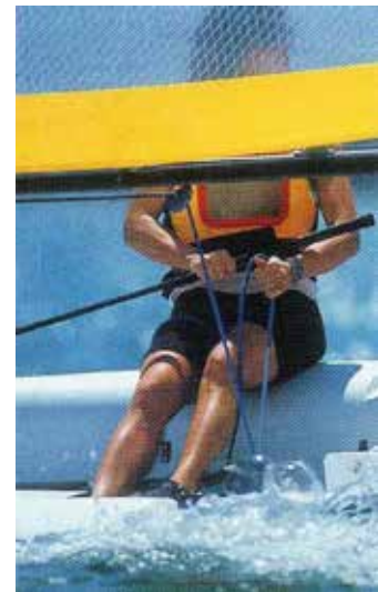
In a boat with a centre mainsheet, hold the tiller extension in a dagger grip with the end across your body. 当主帆索系在船中央时，采用握匕首的方式握住副舵柄，且使其末端在你前面穿过，整个副舵柄置于你的身体之前。
