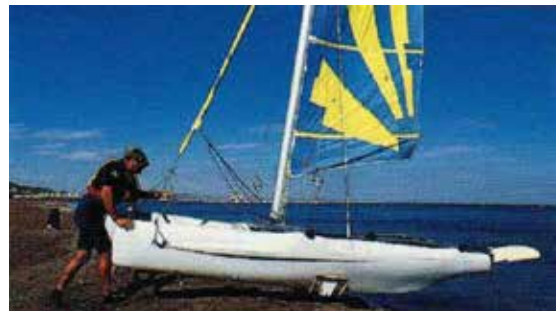
Catamarans use an axle with two wheels and hull supports – hold the bows to push the boat. 双体船的船车由轮轴、两个轮子和船体支架构成。下水时，抓住船头，将船推入水中。
