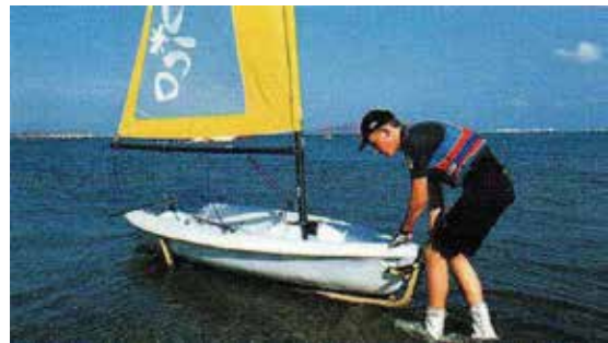
Push the boat into deeper water until it floats off its trolley. 把船推向更深的水域，直至船脱离船车。
