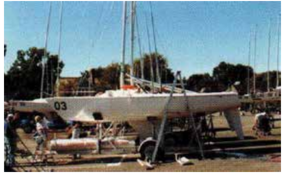
The Sonar has a fixed keel that requires a special cradle or trailer for storage ashore, but it has a simple dinghy-like layout.
