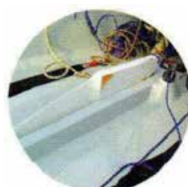
Centreboard pivots up or down to act as a keel. 稳向板上下移动，充当的龙骨。
