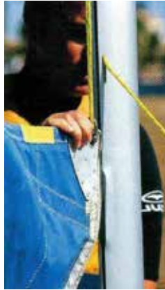
Step 1 Feed the luff into the mast groove and pull on the halyard. 第一步，将帆前缘插入主帆凹槽，然后拉升降索。
