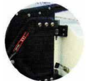
Rudder attaches to boat's transom and is removeable. 船舵卡在船的舵板上，可拆卸。
